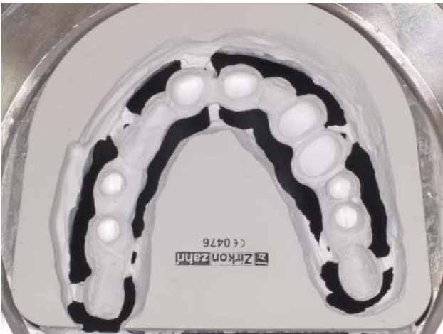
Figure 5. The milled frame at the "green" stage.
